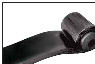
polyurethane bushing in rear eye
