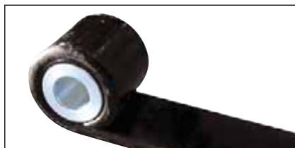
aluminum bushing in front eye
